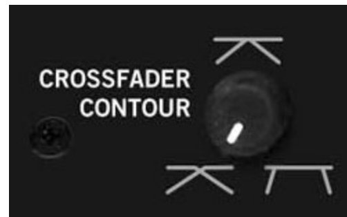
Crossfader Curve Control
